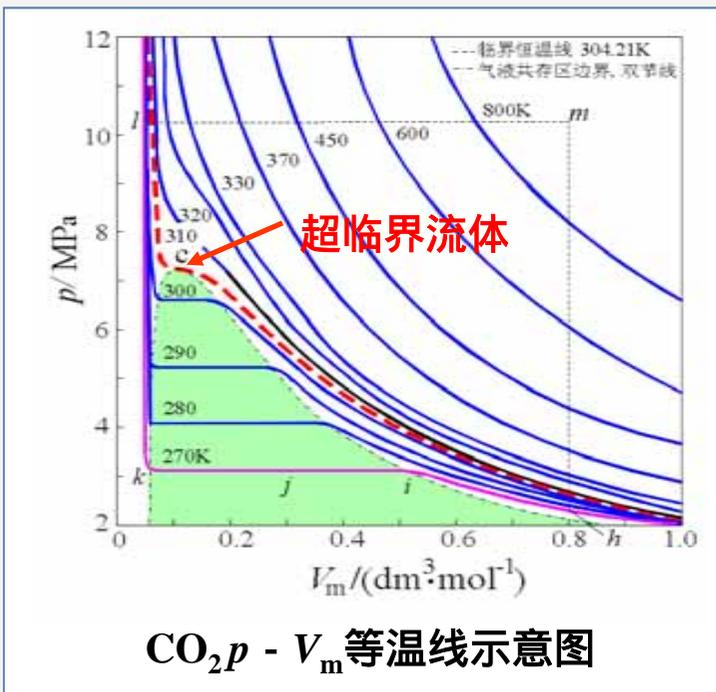
$$\text{CO}_2 : T_c = 31.1 \quad , \quad p_c = 7.28 \text{ MPa}$$
